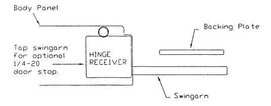
Perform final welding after door has been checked for proper operation.
