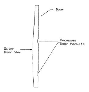
IMPORTANT Tac-weld the door to the body with the desired door gap before attaching the swing arm to the inner door skin. After door has been temporarily attached, push the swing arm up to the inner door skin from inside the vehicle. At this point, mark the holes to be drilled for mounting the door. Slightly over size the mounting holes to allow for future adjustment. Cut door loose and check swing.
