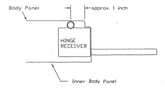
MPSTAIT Notice on the last diagram, the pivot point rests on the outer door skin and is kept back approx. 1" from the door jamb. These two placements are critical. If this placement is not possible in your situation, locate the hinge as close to it as possible.
