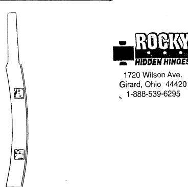
Hold hinge assembly to door jamb and cut out square holes as shown.
