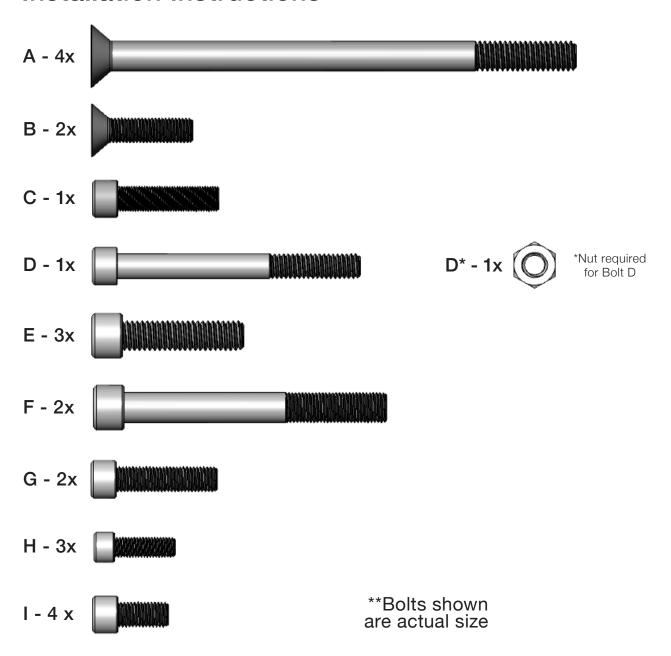
Note: When mounting any of the specified bolts to the engine, Speedmaster recommends that they be installed with some type of sealant such as Loctite #242. This is to overcome the high vibration ranges which the components are subjected to. Tightening torque's of 20 ft./lbs. or 5/16" bolts, 30 ft./lbs. For 3/8" bolts and 40 ft./lbs. for 7/16" bolts are recommended. Please refer to the exploded views in each step for the overall assembly of this serpentine pulley kit.
