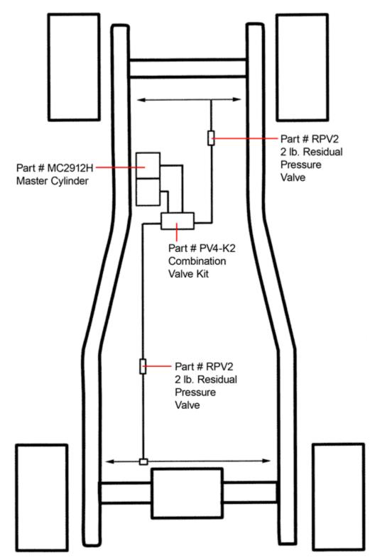
Note: For disc/disc above the floor eliminate RPV2's.
