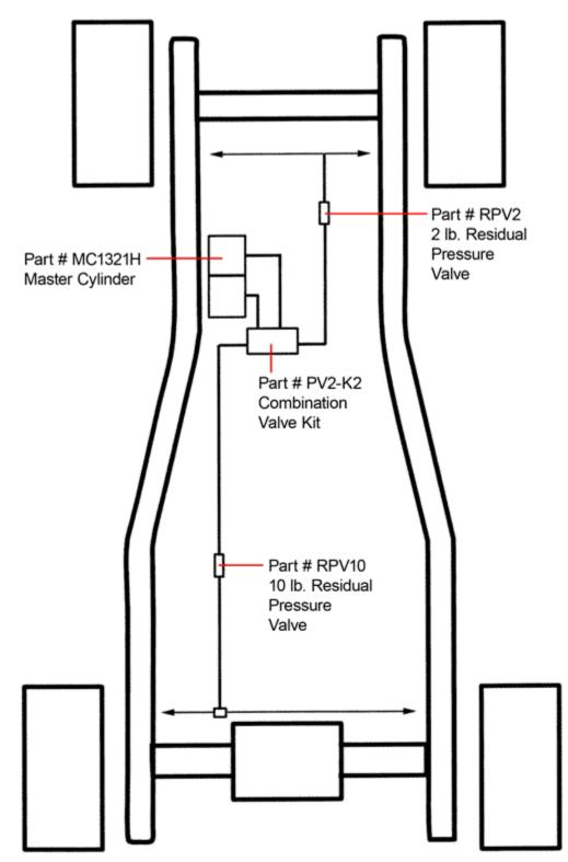
Note: For disc/drum above the floor eliminate RPV2.
