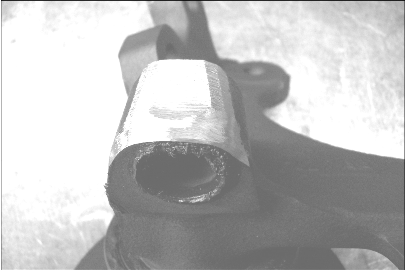
Figure 9 another view of grinding on spindles lower ball joint boss
