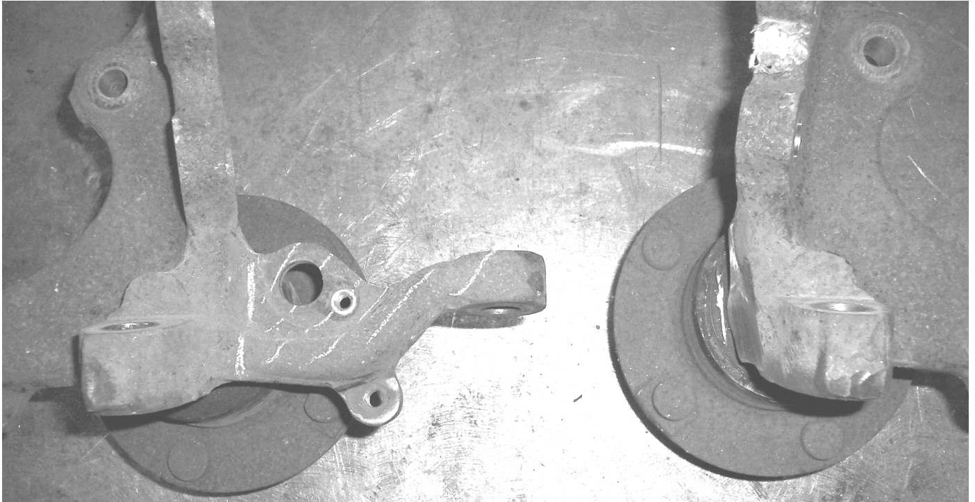
Figure 6 before.....after removing original steering arm from 94-04 spindles
