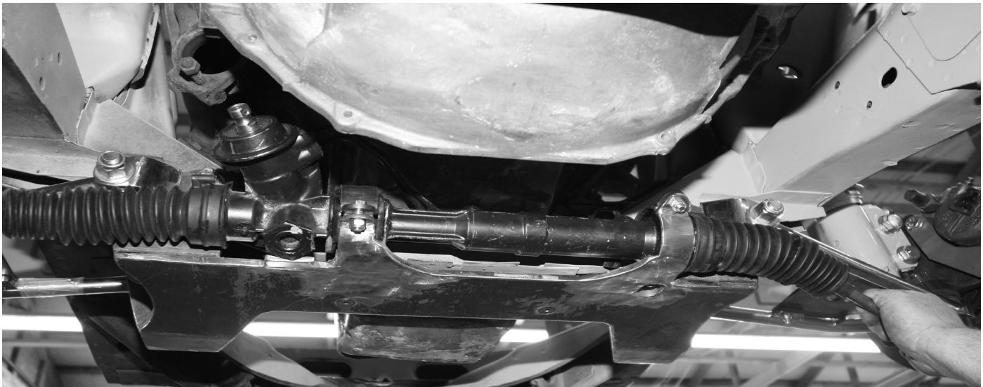
Tightening the driver side upper rack mount bolt with a 1/4" socket, universal, and extension
