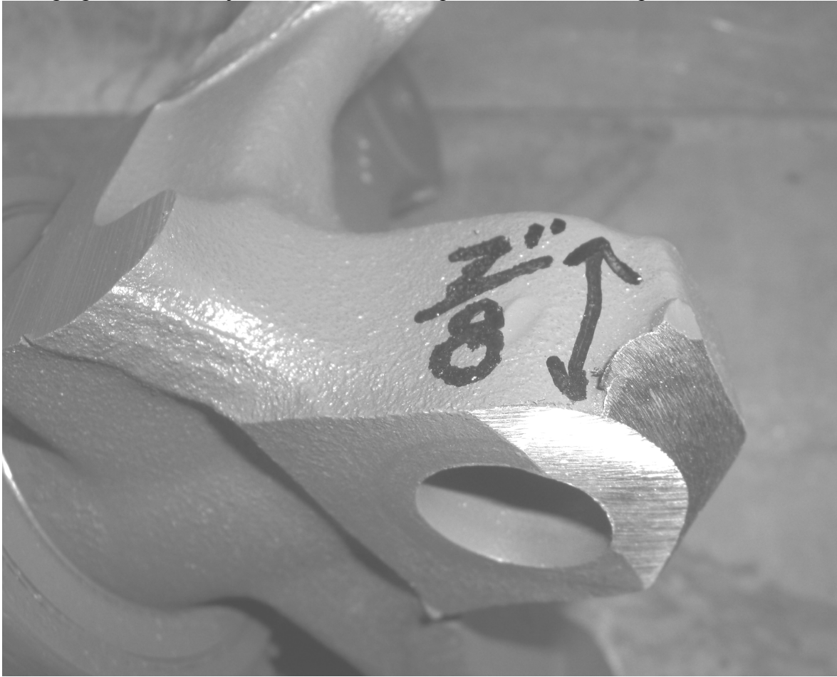
Figure 8 grind bottom of spindle back to 7/8" height on the inboard side
