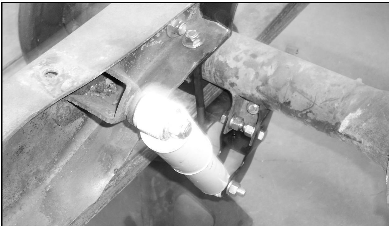
65-69 shock absorber shown, 70-79 has a stud type upper mount on the original frame
