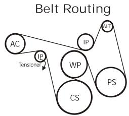
\*BELT DISCLAIMER: The belt included in this bracket kit is designed for standard 105 amp. Alternator applications. If your application is using the optional high output 130-145 amp. alternator; a smaller idler pulley at the factory alternator mount will be necessary for proper fitment of the included 6 rib belt (SEE ALTERNATOR DIMENSIONS ON FRONT PAGE). This smaller idler pulley is readily available at any auto parts store listed under part numbers:
